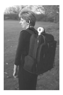
Figure 1. The backpack for running the prototype AudioGPS system and collecting experimental data. The fan-cooled, temperature-monitored backpack contains a laptop connected to a GPS system. The snorkel sticking out of the backpack doubles as a filtered air inlet for the cooling fan and a mounting point for the GPS antenna to optimise GPS signal quality. The laptop is wireless networked to allow it to be monitored remotely by an experimenter when appropriate.
